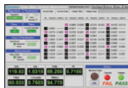
IEC 61000-3-2 Current Harmonic Test (Pre-compliance)
