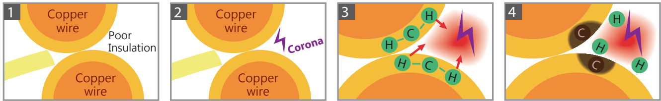
Corona discharge causes insulation layer carbonization
