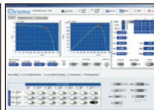
Static MPPT Test
