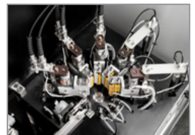
Five layer short test stations
