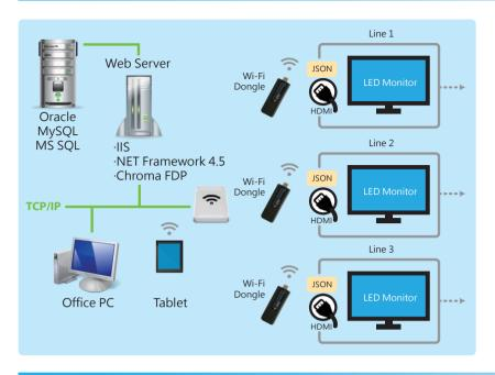
The new generation of Chroma eKanban solution integrates HDMI interface and different kinds of digital display monitors under Android platform. It helps to deliver real-time information to display monitors through Wi-Fi in factories. Moreover, it is easy to set up the layout configuration on Web interface so as to upload and broadcast real-time kanban information to factories, hospitals, retail stores, and public environments, providing the best choice of visual management solution.
