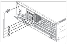
One A330101 power supply supports up to 200W (4 pcs of 33010 digital IO cards)
